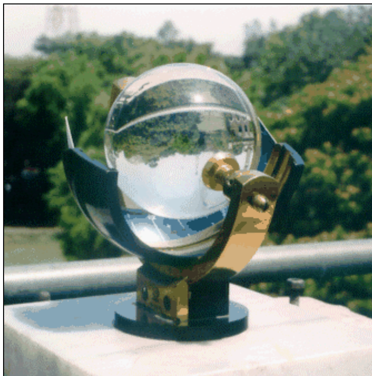
Figure 6.5: Campbell-Stokes sunshine recorder (Latitude 5°S to 45°N)
