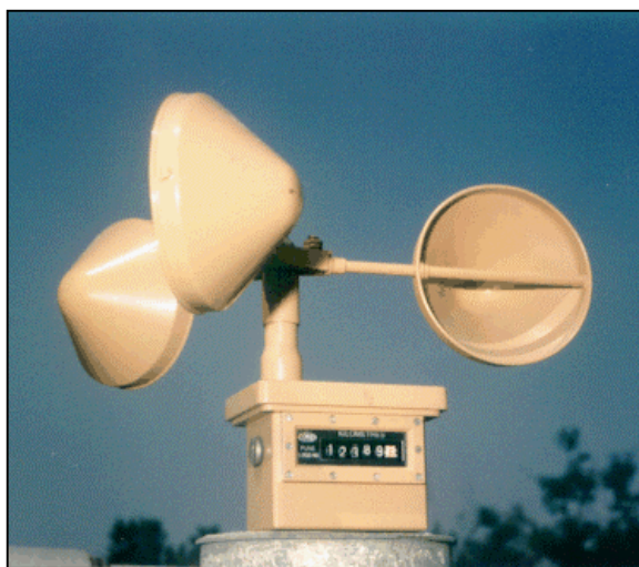
Figure 6.11: General arrangement of cup counter anemometer
