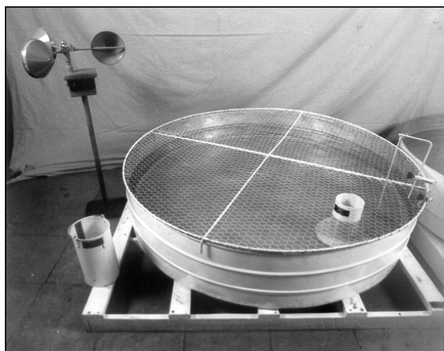
Figure 6.13: US Class A pan evaporimeter, general set up
