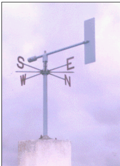
Figure 6.12: General arrangement of wind vane
